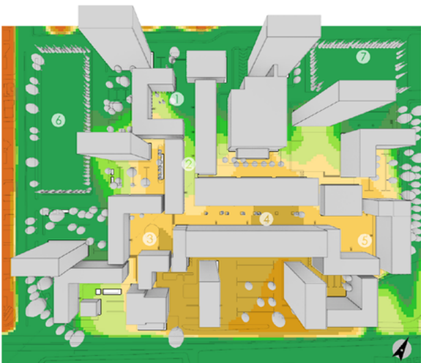
SCENARIO 3: GREEN FACADE AND ROOF PM2.5 concentration at 1.75m above ground level
