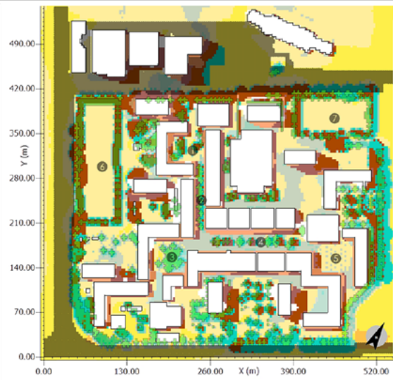
SCENARIO 5: COMBINING SCENARIO 1 + 2 + 3 IMPROVED URBAN VEGETATION + MATERIALS + GREEN FACADES & ROOF UTCI at 1.5m above ground level MIN: 36.58°C MAX: 46.43°C
